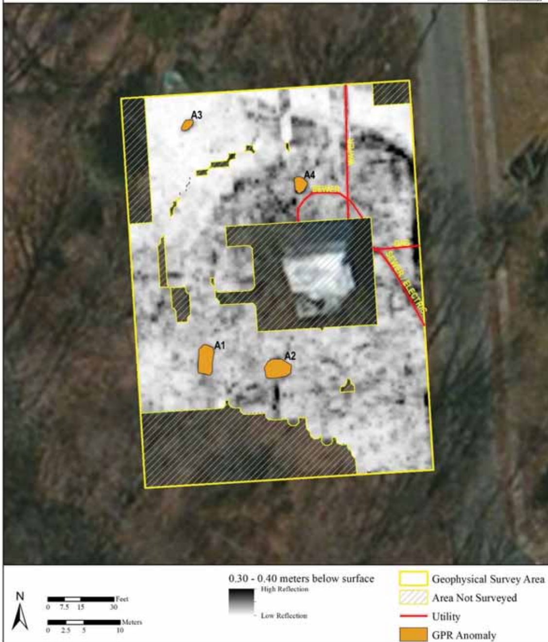
Figure 4-1: Plan view time slice map showing all GPR survey anomalies found at full radar depth range (ESRI 2023).
