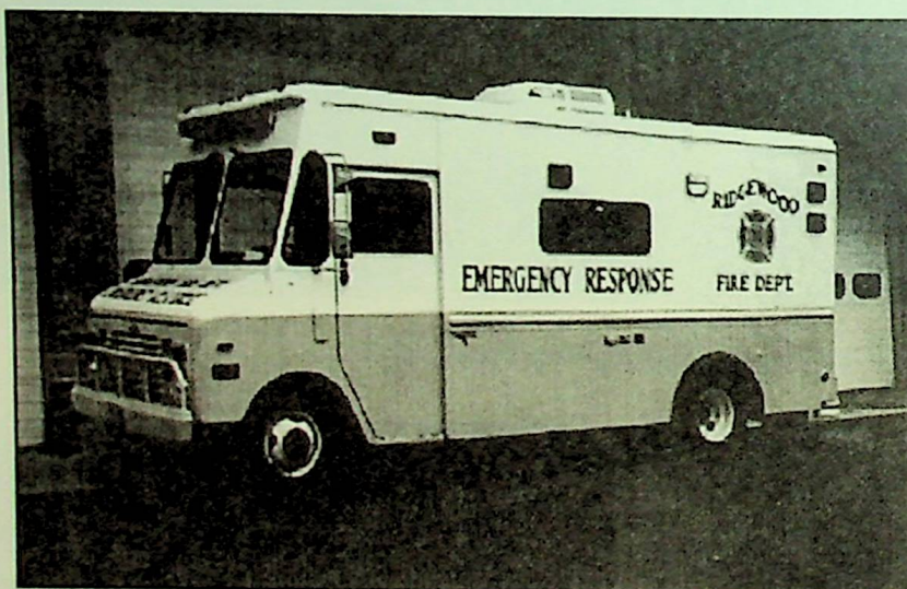
1988 Chevrolet Step Van Emergency Response Unit. This truck carries hazardous material equipment, scuba gear, and a mobile radio communications station. Currently #34.
