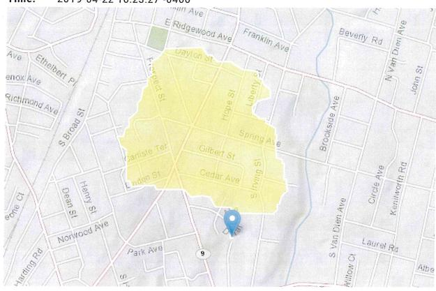
The Stream Stat Mapping Does not account for the fact that the drainage area east of South Maple Avenue is intercepted by the South Maple Avenue drainage system and piped to the Ho- Ho- Kus Brook via the South Maple Avenue-Clayton Street-Southern Parkway storm sewer system, ultimately discharging to the main channel of Ho-Ho-Kus Brook via a 48" RCP well north of Hopper Ridge See original Hopper Ridge Townhomes Drainage Area Plan by Andrew Marshall, dated 6/24/82.
